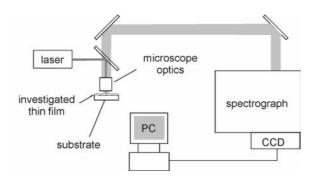
Fig. 2. Micro-Raman system using backscattering configuration
