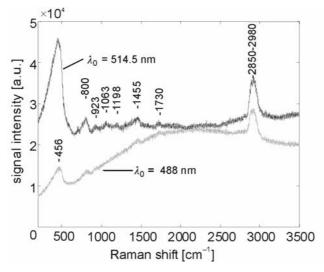
Fig. 3. Raman spectra of samples based on systems of GPTS and MPTS, recorded at various excitation wavelengths  $\lambda_0$
