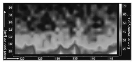
Fig. 6. The image of the edge of an investigated thin-film structure recorded using Raman mapping of the line assigned to C–H bonds
