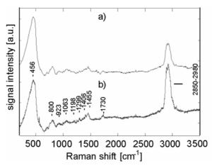
Fig. 4. Micro-Raman spectra of thin films based on systems of GPTS and MPTS; thickness: a) 3  $\mu$ m, b) 4  $\mu$ m
