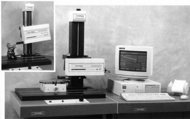
Fig. 3. Stand for stereometric investigations of surface (Taylor Hobson's profilographometer)
