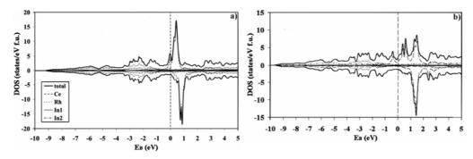
Fig. 4. Total and partial spin up and spin down DOSs for CeIrIn<sub>5</sub> calculated by: GGA (a) and by GGA + SO + U (1.75 eV) (b)
