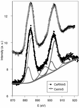
Fig. 2. Ce 3d XPS spectra for CeRhIn $_5$  and CeIrIn $_5$ . For CeRhIn $_5$ , separated and overlapping peaks attributed to the  $4d^9f^2$ ,  $4d^9f^1$  and  $4d^9f^0$  final states are also shown
