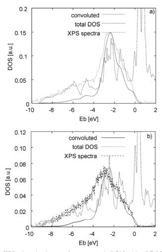
Fig. 1. XPS valence band spectra for paramagnetic  $CeRhIn_{5}\left(a\right)$  and  $CeIrIn_{5}\left(b\right)$
