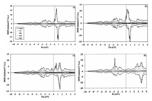
Fig. 3. Total and partial spin up and spin down DOSs for CeRh $In_5$  calculated by the following methods: GGA (a), GGA + SO (b), GGA + SO + U (1.65 eV) (c) and GGA + SO + U (6.8 eV) (d)
