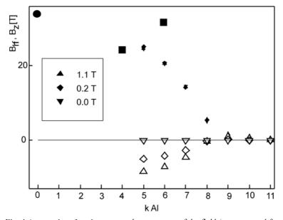
Fig. 4 Average h.m.f. and average z-th component of the field (not corrected for the external field) related to the sectors from Fig. 2, under the assumption that contributions from the first and the second coordination shells to the h.m.f. are the same. Full symbols correspond to the h.m.f., open symbols to the z-component of the h.m.f., • − Ref [16], ■ − Ref. [29]
