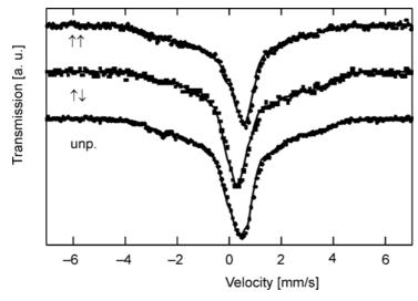
Fig. 1. An example of the Mössbauer spectra recorded at T=13 K with polarized and unpolarized radiation in an axial, externally applied magnetic field of 1.1 T. The arrows  $\uparrow \uparrow$  and  $\uparrow \downarrow$  indicate two opposite circular polarizations. Solid lines represent the results of the simultaneous fitting the h.m.fs to all the recorded spectra
