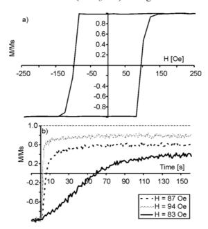
Fig. 1. Magnetic hysteresis loop for a cobalt film with a thickness of d = 1.5 nm (a) and time dependences of film magnetization for different strengths of the applied magnetic field (b)
