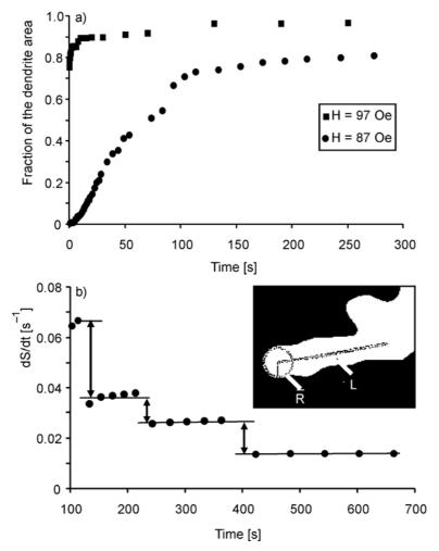
Fig. 3. Time dependence of the total reversed area fraction of domains for two amplitudes of the magnetic field (a) and time derivative of dendrite area (b), H = 87 Oe. The inset shows the geometry of a dendrite finger
