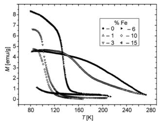
Fig. 1. Temperature dependence of magnetisation for La<sub>0.67</sub>Ca<sub>0.33</sub>Mn<sub>1-x</sub>Fe<sub>x</sub>O<sub>3</sub> with a given x in a magnetic field of 100 Oe
