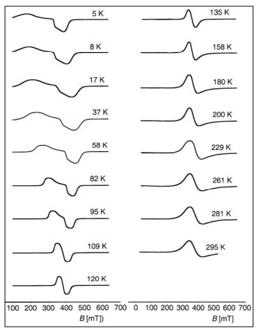
Fig. 3. Temperature dependence of the ESR spectra of  $La_{0.67}Ca_{0.33}Mn_{1-x}Fe_xO_3$  for x = 0.1
