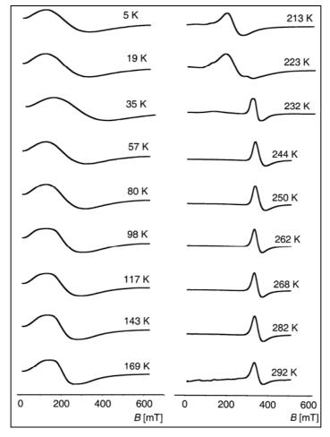
Fig. 2. Temperature dependence of the ESR spectra of  $La_{0.67}Ca_{0.33}Mn_{1-x}Fe_xO_3$  for x = 0
