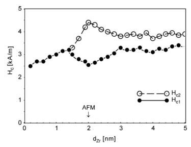
Fig. 2. Two different coercive fields  $H_{c1}$  and  $H_{c2}$  as functions of Zr interlayer thickness for a wedged 20 nm Fe/ $d_{\rm Zr}$  Zr/20 nm Fe trilayer
