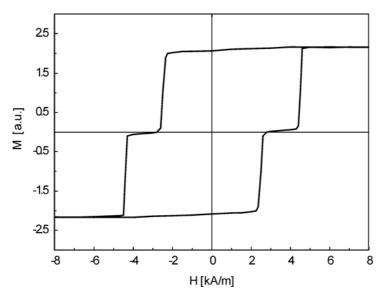
Fig. 1. A hysteresis loop of the 20 nm -Fe/2 nm - Zr/20 nm - Fe trilayer
