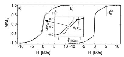
Fig. 1. Exemplary hysteresis loops of MLs with  $t_{\rm Co} = 0.8$  nm and  $t_{\rm Au} = 2.2$  nm, at room temperature in perpendicular (a) and parallel (b) configurations of the applied field
