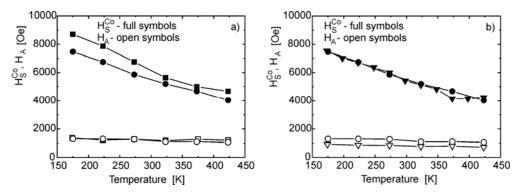
Fig. 2. Temperature dependence of the  $H_s^{Co}$  and  $H_A$  fields in the MLs:
