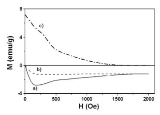
Fig. 4. Simultaneous measurement of two components  $(M_x \text{ and } M_y)$  vs. applied field: a)  $M_x$  (single flux state) along the x-direction (ab-plane), b)  $M_x$  (two flux condition) along the x-direction (ab-plane), c)  $M_y$  (two flux condition) along the y-direction (c-axis),  $H_{FC} = 1$  kOe and T = 77 K
