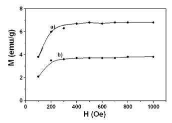
Fig. 2. Remnant moment against cooling field  $H_{FC}$  for the field along: a) the c-axis  $(M_{\rm rem}^c)$ , b) along the ab-plane  $(M_{\rm rem}^{ab})$
