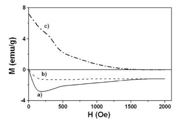
Fig. 1. M(H) loops of YBa<sub>2</sub>Cu<sub>3</sub>O<sub>7-x</sub> at T = 77 K in zero field cooling condition: a) along *c*-axis, b) along *ab*-plane
