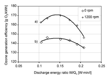
Fig. 6. Ozone generation efficiency for various electrode rotational speeds vs. discharge energy ratio: a) setup 1, gas gap: 1.5 mm, flow: 1.5 dm³/min b) setup 2, gas gap: 3.0 mm, gas flow rate: 3.0 dm³/min
