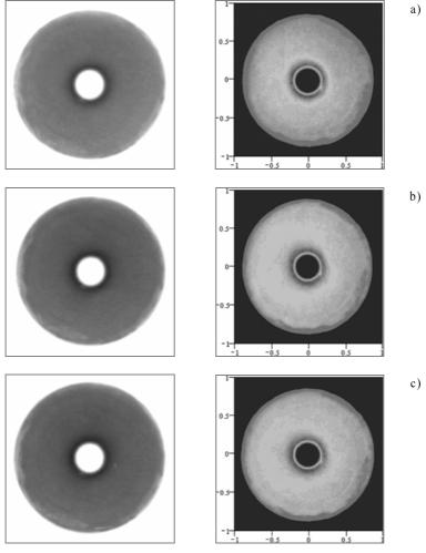
Fig. 5. Discharge photo- and computer analysis. Gas gap -0.5 mm; gas - oxygen, flow -1.5 dm $^3$ /min, voltage -9.0 kV, dielectric - glass (0.75 mm), rotational speed: a) 0 rpm, b) 1200 rpm; c) 1600 rpm
