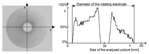
Fig. 4. Discharge picture with the analysis of discharge intensity
