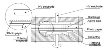
Fig. 3. Scheme of the discharge photography method
