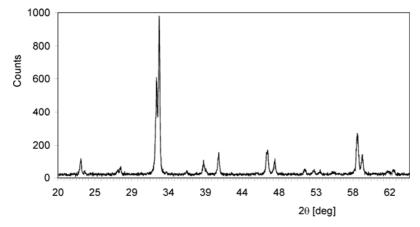
Fig. 5. XRD pattern for standard  $YBa_2Cu_3O_{7-\!\delta}$
