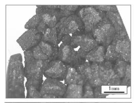
Fig. 1. Sample obtained by mixing  $YBa_2Cu_3O_{7-\delta}$  granules of the size of 0.63 – 0.8 mm, not pressed and sintered at 950 °C by 3h
