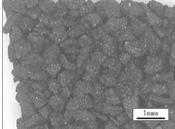
Fig. 2. Sample obtained by sintering YBa<sub>2</sub>Cu<sub>3</sub>O<sub>7-δ</sub> granules filled with wax and slightly pressed
