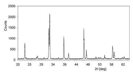
Fig. 6. XRD pattern for the YBa<sub>2</sub>Cu<sub>3</sub>O<sub>7-δ</sub> after sintering with sugar
