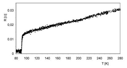
Fig. 7. R-T plot for a superconductive sample having open pores filled with Iron and fixed with wax
