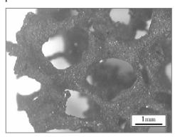
Fig. 3. A porous sample obtained by burning out PPI foams covered with YBa<sub>2</sub>Cu<sub>3</sub>O<sub>7-\delta</sub> suspension
