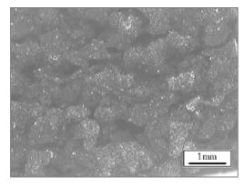
Fig. 4. The outer side of the porous sample  $YBa_2Cu_3O_{7-\delta}$  and sucrose granules pressed at 700 MPa sintered at 935 °C by 36 h and oxidized at 475 °C by 36 h
