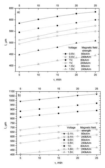
Fig. 5. Time dependences of the cavity length l of the quasi-periodic surface structure of the cylinder: a) under its cathode corrosion in 7% solution of nitric acid, b) under its anode corrosion. Mean error  $\sim 25\%$
