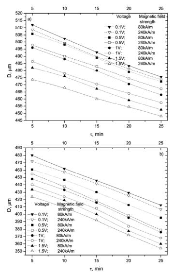
Fig. 7. Time dependences of the cylinder diameter D at the elevation of the quasi-periodic surface structure of the cylinder: a) under its cathode corrosion b) under its anode corrosion in the 7% solution of nitric acid. Mean error  $\sim 25\%$
