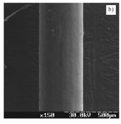
Fig. 2. An iron cylinder after corrosion in 14% solution of nitric acid, the voltage between the cylinders is 1.5 V, the duration of experiment – 10 min: a) cathode corrosion; b) anode corrosion
