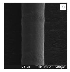
Fig. 3. An iron cylinder after corrosion in 14% solution of nitric acid, the voltage between the cylinders is 1.5 V, the magnetic field strength – 240 kA/m, the duration of experiment – 10 min: a) cathode corrosion; b) anode corrosion
