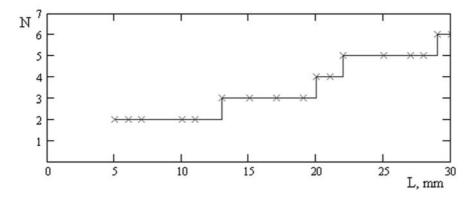
Fig. 4. Dependence of the number of vortexes on the cylinder length L. Cylinder diameter is equal to 0.725 mm (the experimental points are marked with  $\times$ )
