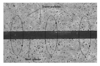
Fig. 1. Schematic drawing of the multivortex structure in the vicinity of a steel cylinder in a steady magnetic field (1, 2, 3 – electrolyte vortexes)
