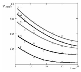
Fig. 2. Vortex velocity dependence on magnetic field magnitude in the vicinity of the steel cylinder surface. The magnetic field H: 1-1000 Oe, 2-2000 Oe, 3-3000 Oe, 4-4000 Oe; 5-500 Oe
