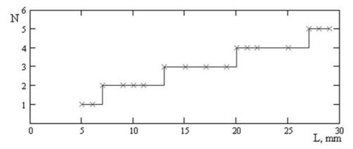
Fig. 5. Dependence of the number of vortexes on the cylinder length L. Cylinder diameter is equal to 0.250 mm (the experimental points are marked with  $\times$ )
