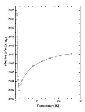
Fig. 4. Temperature dependence of the  $g_{\text{eff}}$  parameter
