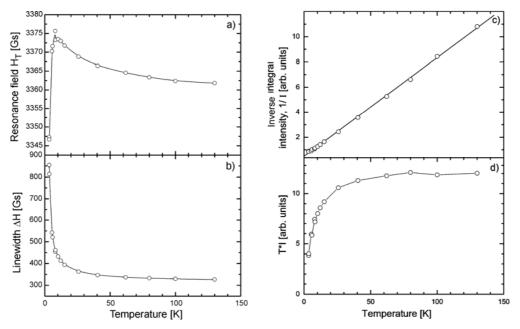
Fig. 3. Temperature dependence of the ESR resonance field (a), linewidth (b), inverse integral intensity (c) and the product of the integral intensity and temperature (d)
