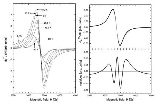
Fig. 1. Temperature dependence of the ESR spectra of the CH<sub>2</sub>(COOH)<sub>2</sub>·MnCO<sub>3</sub>·H<sub>2</sub>O complex
