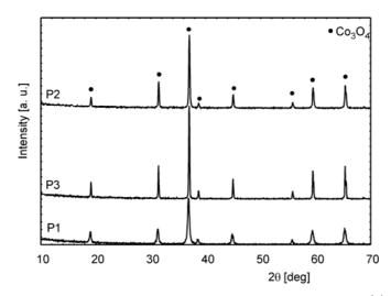
Fig. 2. XRD patterns for the three investigated samples of Co<sub>3</sub>O<sub>4</sub> particles
