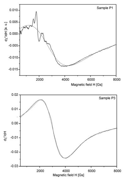
Fig. 4. The fitted (dotted lines) and experimental (solid lines) EPR spectra of sample P1 and sample P3
