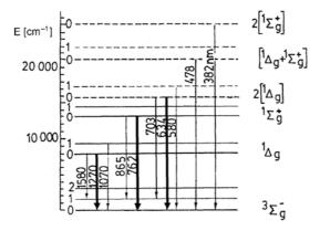
Fig. 7. Scheme of energetic levels and electronic transitions in singlet oxygen molecules [32]
