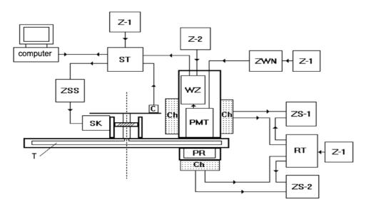
Fig. 1. Scheme of the filter spectrometer: PR – sample, T – turning round shield with cut-off filters, SK – stepping motor, C – controller of start position, PMT – photomultiplier, Ch – thermoelectric cooler, WZ – pulse amplifier, Z, ZS, ZWN, ZSS – voltage supplies, ST – interface, RT – temperature controller
