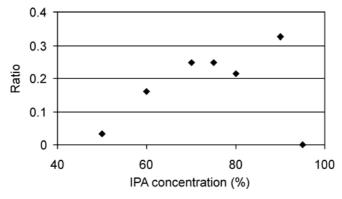
Fig. 6. The ratio of etching rates of (111) and (100) planes vs. [IPA] concentration: [TMAH] – 0.83%, 60 °C, 3h
