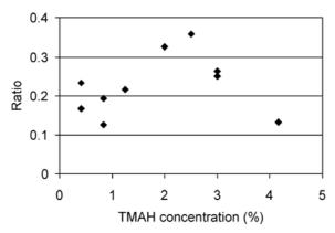
Fig. 5. The ratio of etching rates of (111) and (100) planes vs. TMAH concentration: [IPA] - 83%, 60 °C, 3h
