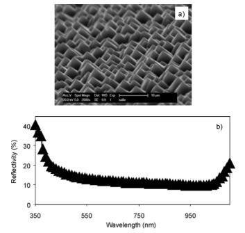
Fig. 1. SEM picture (a) of a TMAH textured wafer after optimized etching (30 min, 2% TMAH, 10% IPA, 80 °C). Hemispherical reflectance (b) of a TMAH textured silicon sample (30 min, 2% TMAH, 9% IPA, 90 °C)
