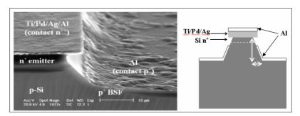
Fig. 3. Scanning electron microscopy picture (left) of a self-aligned interdigitated back-contact solar cell and of the Ti/Pd/Ag cantilever obtained by TMAH etching. Structure (right) of a self-aligned interdigitated back-contact solar cell (only one contact has been shown). The vertical white arrow corresponds to the etch depth ((100) planes) and the horizontal one to the etch width ((111) planes)
