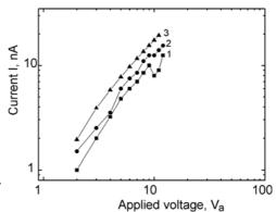
Fig. 4. Room-temperature experimental (1, 2) and calculated (3) current-voltage characteristics of NaSbSe<sub>2</sub> films deposited onto the "cold" substrate
