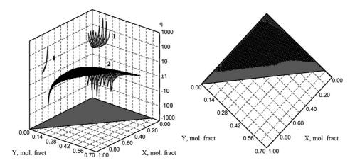
Fig. 2. Stabilization factor of  $Ga_xIn_{1-x}P_yAs_zSb_{1-y-z}/InAs$  system at 773 K, f = -1%. (111): 1 - p ositive values, 2 - n egative values
