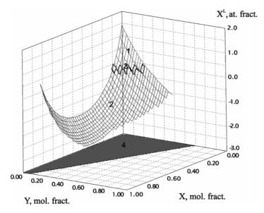
Fig. 1. Contact supercooling in  $Ga_xIn_{1-x}P_yAs_zSb_{1-y-z}InAs$  system at 773 K, f = -1% (111): 1 – positive values, 2 – negative values, 3 – the range of circumzero values, 4 – a projection of the isoperiodic section
