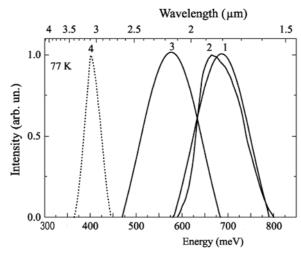
Fig. 5. PL spectra of  $Ga_{0.92}In_{0.08}P_{0.05}As_{0.08}Sb_{0.87}/InAs$  heterostructure: 1 – undoped, 2 – Zn-doped, 3 – Te-doped, 4 – InAs substrate
