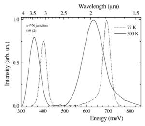
Fig. 6. EL spectra of the n-InAs/P-GaInPAsSb/N-GaInPAsSb structure
