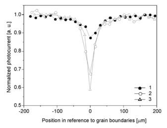
Fig. 1. The cross-section of the current signal across the interface of grains for the cells with  $SiN_x$ :H (1 – IMEC, 2 – AGH) and the reference cell with  $TiO_x/SiO_2$  (3)
