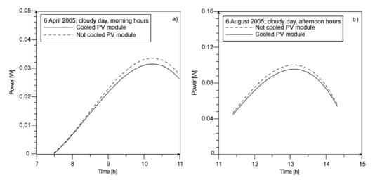
Fig. 3. Power generated in PV modules at a cloudy day in: a) morning and b) afternoon hours
