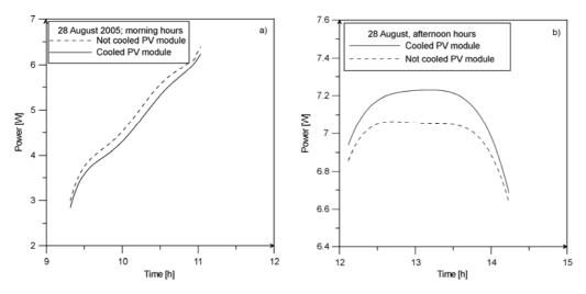
Fig. 1. Power generated in PV modules in a sunny day, in the morning (a) and afternoon (b)
