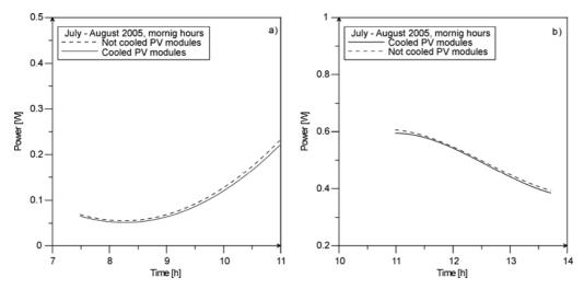
Fig. 4. Average power generated in PV modules in cloudy days of July and August 2005, in the morning (a) and afternoon (b)
