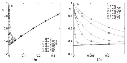
Fig. 3. The value of Poisson's ratio against the inverse of the exponent n for two-dimensional soft discs with different values of the polydispersity parameter: a)  $n \ge 3$ , b)  $n \ge 96$ . The thick solid line shows the exact result for  $\delta = 0$ , see Eq. (7). The dotted lines are presented to guide the eye
