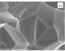
Fig. 2. SEM photographs of the domain structure: a) ceramics with the rhombohedral structure, b) ceramics with the tetragonal structure, c) ceramics from the morphotropic area
