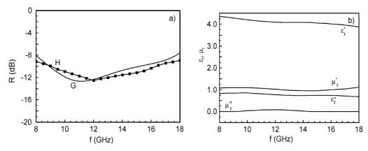
Fig. 8. Reflectivity versus frequency for sample 4 (a): G – experimental results, H – theoretical values,  $\varepsilon_r$  and  $\mu_r$  spectra of the second layer of sample 4 (b)
