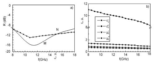
Fig. 10. Reflectivity versus frequency for sample 6 (a): M – experimental results, N – theoretical values,  $\varepsilon_r$  and  $\mu_r$  spectra of the second layer of sample 6 (b)
