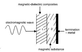
Fig. 4. Structure of a two-layer wave absorber
