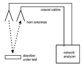
Fig. 5. Schematic diagram of the experiment system
