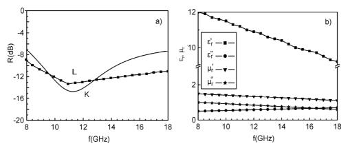
Fig. 9. Reflectivity versus frequency for sample 5 (a): K – experimental results, L – theoretical values, the  $\varepsilon_r$  and  $\mu_r$  spectra of the second layer of sample 5 (b)
