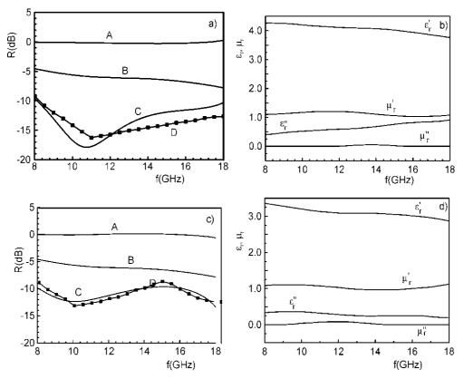
Fig. 6. Reflectivity versus frequency for sample 1 (a),  $\varepsilon_r$  and  $\mu_r$  spectra of the second layer of sample 1 (b), reflectivity versus frequency for sample 2 (c),  $\varepsilon_r$  and  $\mu_r$  spectra of the second layer of sample 2 (d); A – reflectivity of the second layer, B – reflectivity of the first layer, C – experimental results, D – theoretical curves
