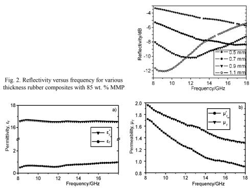
Fig. 3. Relative permittivity (a) and relative permeability (b) as functions of frequency for the rubber composites with 85 wt. % MMP
