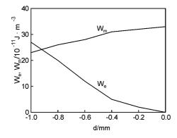
Fig. 1. Distribution of energy density in absorbing materials
