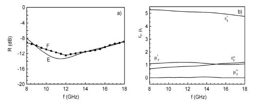
Fig. 7. Reflectivity versus frequency for sample 3 (a): E – experimental results, F – theoretical values,  $\varepsilon_r$  and  $\mu_r$  spectra of the second layer of sample 3 (b)
