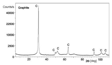
Fig. 6. X-ray diffractogram of graphite
