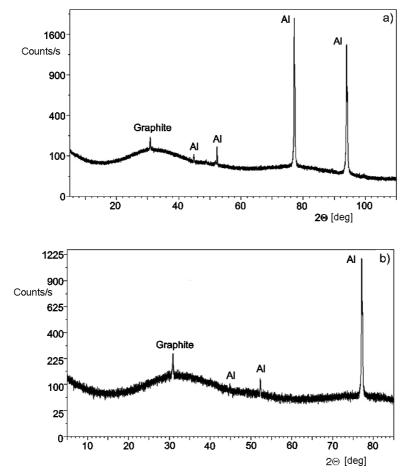
Fig. 5. X-ray diffractograms of the composite layers for samples: a) 4C, b) 4D
