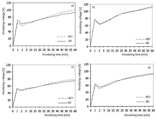
Fig. 9. Relations between anodizing voltage, time of process and composition of electrolyte and temperature for samples: a) 4A1, 4A, b) 4B1, 4B, c) 4C1, 4C, d) 4D1, 4D
