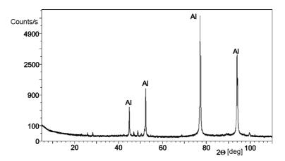
Fig. 3. X-ray diffractogram of the AlMg<sub>2</sub> alloy
