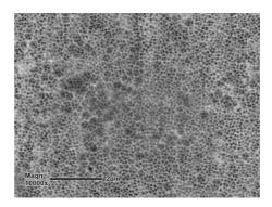
Fig. 2. Morphology of the oxide layer surface obtained at 293 K and current density of 2 A/dm<sup>2</sup>
