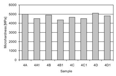
Fig. 8. Effect of anodizing conditions on microhardness of oxide and composite layers
