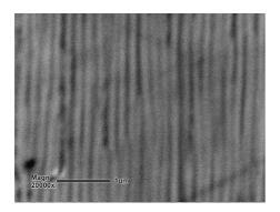
Fig. 1. Structure of the oxide layer obtained at 293 K and current density of 2 A/dm<sup>2</sup>
