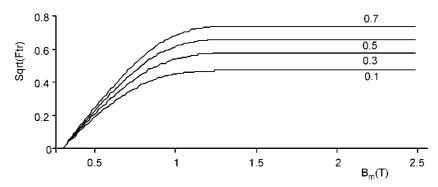
Fig. 7. Influence of filling the ceramic superconductor with grains on the square root of the flux trapped [Sqrt(Ftr)] versus maximum magnetic field in a cycle
