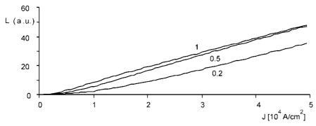
Fig. 2. Dependence of the value of losses on the transport current density for three nickel substrate magnetic characteristics described by Eq. (1);  $B \propto 0.65 \tanh(\beta \mu_0 H)$  for  $\beta = 0.2, 0.5, 1$
