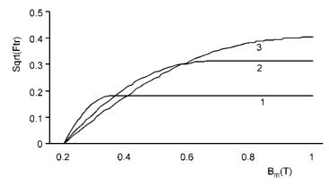
Fig. 8. The influence of the intergranular critical current density of the ceramic superconductor on a square root of the flux trapped [Sqrt(Ftr)] versus maximum magnetic field in the cycle.
