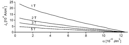
Fig. 5. Dependence of the critical current density on the elasticity force of the vortex lattice (described by the parameter *J*) versus magnetic induction for pinning centre concentration equal to  $2 \times 10^{14}$  cm<sup>-3</sup>
