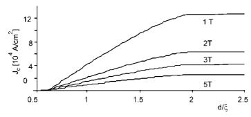
Fig. 4. Dependence of the critical current density satisfying the electric field criterion on the pinning centre dimensions for various magnetic fields; pinning centre concentration equal to  $2 \times 10^{14}$  cm<sup>-3</sup>
