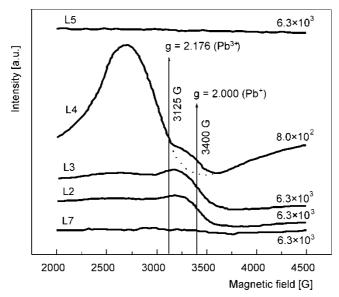
Fig. 4. Room temperature EPR spectra of L2–L5 and L7 glasses (receiver gain is given inside the figure at the right hand side)
