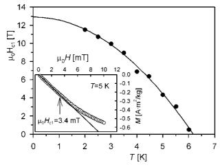
Fig. 5. The lower critical field  $H_{\rm cl}(T)$  corrected for the demagnetising effect. The inset shows the magnetisation versus applied magnetic field M(H) for 5 K and the criterion for determination of  $H_{\rm cl}(T)$ . The data in the inset are as measured (not corrected)
