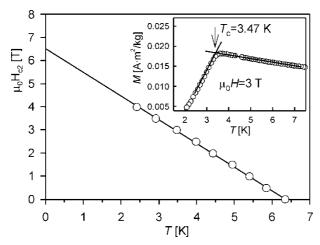
Fig. 4. Upper critical field  $H_{c2}(T)$  for  $Mo_2Re_3B_x$ – $Mo_3Re_2B_x$  eutectic. The inset presents the way of determination of the critical temperature  $T_c(H)$  for a selected magnetic field (3 T in this case)
