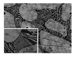
Fig. 1. The SEM micrography of  $Mo_2Re_3B_x$ — $Mo_3Re_2B_x$  sample. Inset: the example of regular lamellar structure between globules of  $Mo_3Re_2B_x$  phase
