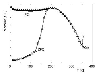
Fig. 3. FC (solid symbols) and ZFC (open symbols) M(T) dependences for the  $B2/L2_1$  ordered Co<sub>2</sub>CrAl film annealed at 760 K (state 4)
