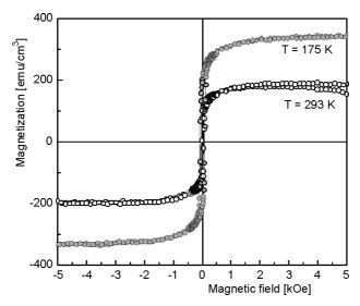
Fig. 2. Magnetization measured at 175 K and 293 K as a function of magnetic field for B2/L2<sub>1</sub> ordered Co<sub>2</sub>CrAl film annealed at 760 K (state 4)
