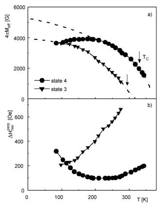
Fig. 4. Temperature dependences of the effective magnetization  $4\pi M_{\rm eff}$  of the Co<sub>2</sub>CrAl films annealed at 608 K (state 3) and 760 K (state 4) (a); FMR resonance linewidth  $\Delta H$  for the same films (b)
