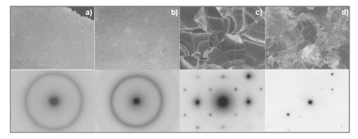
Fig. 1. Room temperature TEM micrographs and diffraction patterns for the  $Co_2CrAl$  films deposited onto NaCl substrates at 150 K (a), annealed at 538 K (b), 608 K (c) and 760 K (d)
