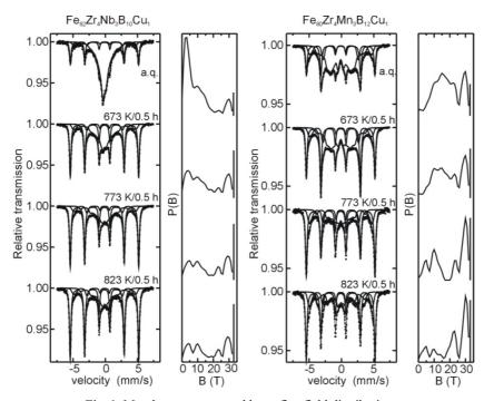
Fig. 1. Mössbauer spectra and hyperfine field distributions of the  $Fe_{82}(Zr_4Nb_3)B_{10}Cu_1$  and  $Fe_{80}(Zr_4Mn_3)B_{12}Cu_1$  alloys
