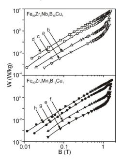
Fig. 3. Dependences of core losses (W) on induction (B) for the Fe<sub>82</sub>(Zr<sub>4</sub>Nb<sub>3</sub>)B<sub>10</sub>Cu<sub>1</sub> alloy (a, b, c, d) and Fe<sub>80</sub>(Zr<sub>4</sub>Mn<sub>3</sub>)B<sub>12</sub>Cu<sub>1</sub> alloy (e, f, g, h) after 0.5 h annealing at 823 K and 773 K, respectively, measured at the frequency of 50 Hz (a, e), 200 Hz (b, f), 1 kHz (c, g), and 2 kHz (d, h)
