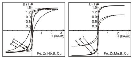
Fig. 2. DC hysteresis loops for the  $Fe_{82}(Zr_4Nb_3)B_{10}Cu_1$  (a, b, c) and  $Fe_{80}(Zr_4Mn_3)B_{12}Cu_1$  (d, e, f) alloys in the as-quenched state (a, d) and after 0.5 h annealing at 773 K (b, e) and 823 K (c, f)
