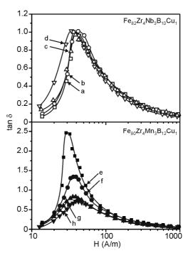
Fig. 5. Dependences of the loss factor ( $\tan\delta$ ) on magnetic field (H) at f=250 Hz for the  $Fe_{82}(Zr_4Nb_3)B_{10}Cu_1$  (a, b, c, d) and  $Fe_{80}(Zr_4Mn_3)B_{12}Cu_1$  (e, f, g, h) alloys in the as quenched state (a, e) and annealed for 0.5 h at 673 K (b, f), 773 K (c, g) and 823 K (d, h)
