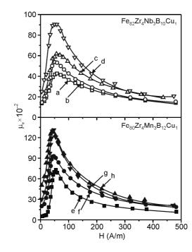
Fig. 4. Effective permeability ( $\mu_e$ ) vs. magnetic field (H) for the Fe<sub>82</sub>(Zr<sub>4</sub>Nb<sub>3</sub>)B<sub>10</sub>Cu<sub>1</sub> (a, b, c, d) and Fe<sub>80</sub>(Zr<sub>4</sub>Mn<sub>3</sub>)B<sub>12</sub>Cu<sub>1</sub> (e, f, g, h) alloys in the as-quenched state (a, e) and annealed at 673 K (b, f), 773 K (c, g) and 823 K (d, h) for 0.5 h measured at the frequency of 250 Hz
