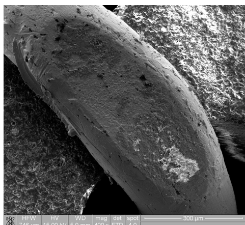
Fig. 2. SEM images of the flattened part of the Au electrode
