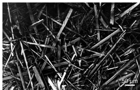
Fig. 6. SEM of K_2Ti_6O_{13} whiskers synthesized by the calcination and slow cooling [31]
