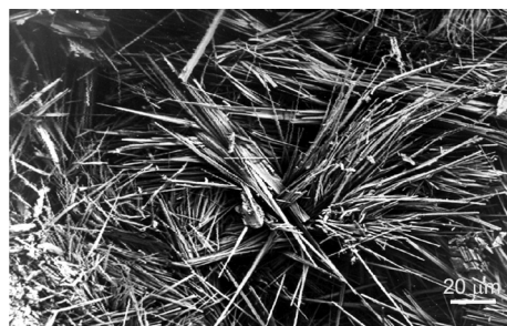
Fig. 4. SEM of K_2Ti_4O_9 whiskers synthesized by the calcination at 1150 °C for 3 h and cooled to 950 °C at the rate of 25 °C·h -1 [29]
