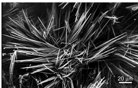
Fig. 3. SEM of K_2Ti_4O_9 whiskers synthesized by the calcination at 1150 °C for 3 h and cooled to 950 °C at the rate of 35 °C·h -1 [29]
