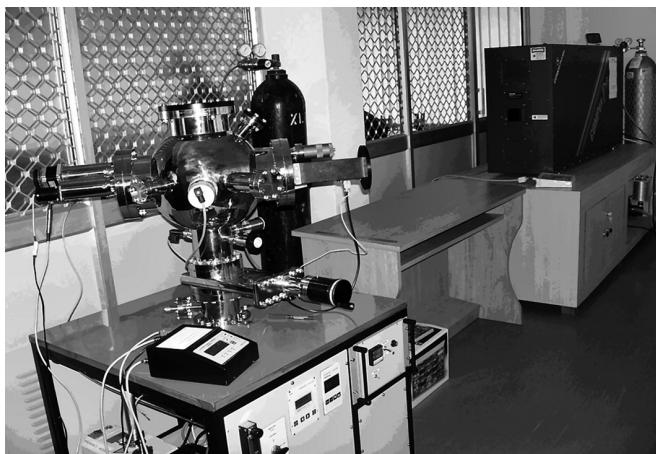
Fig. 1. Complete PLD set up
